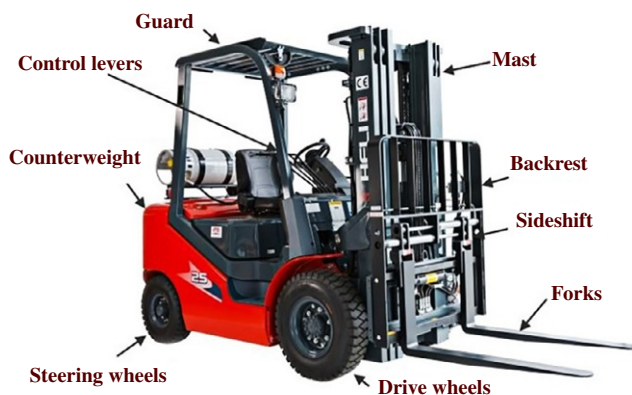
FIG. 12.9 Main components of fork lifts (Cottingham, 2018).
