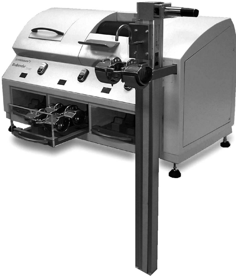
Figure 7 A Brabender Extensograph-E
