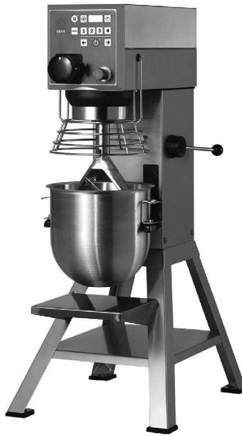
Figure 3 A planetary mixer, used to make cakes, for example
