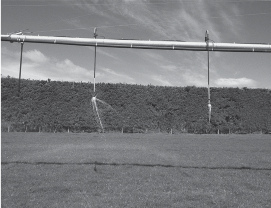
Figure 10.3 Macroirrigator, with organic material (noodle-like material) blocking the nozzles.
