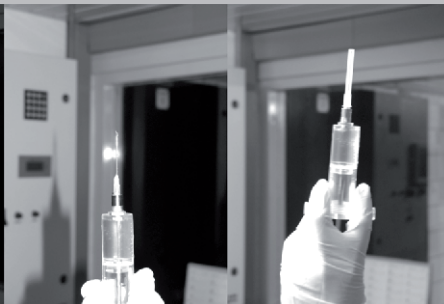
Let some air in the syringe, take the bottle, inject the needle, inject the air in the syringe into the bottle, take the proper volume out of the bottle, eject the last bit of air, put the protection cap on the needle when you are to transport the syringe.
